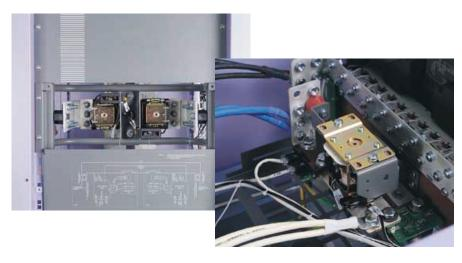
The Intergy range of Low Voltage Disconnect (LVD) modules provide automatic over-discharge protection for valve regulated lead acid (VRLA) batteries. Available in a range of sizes, the units are easily configured from the SM50 or SM30 (with LVD Controller) Intergy Supervisory Modules.
